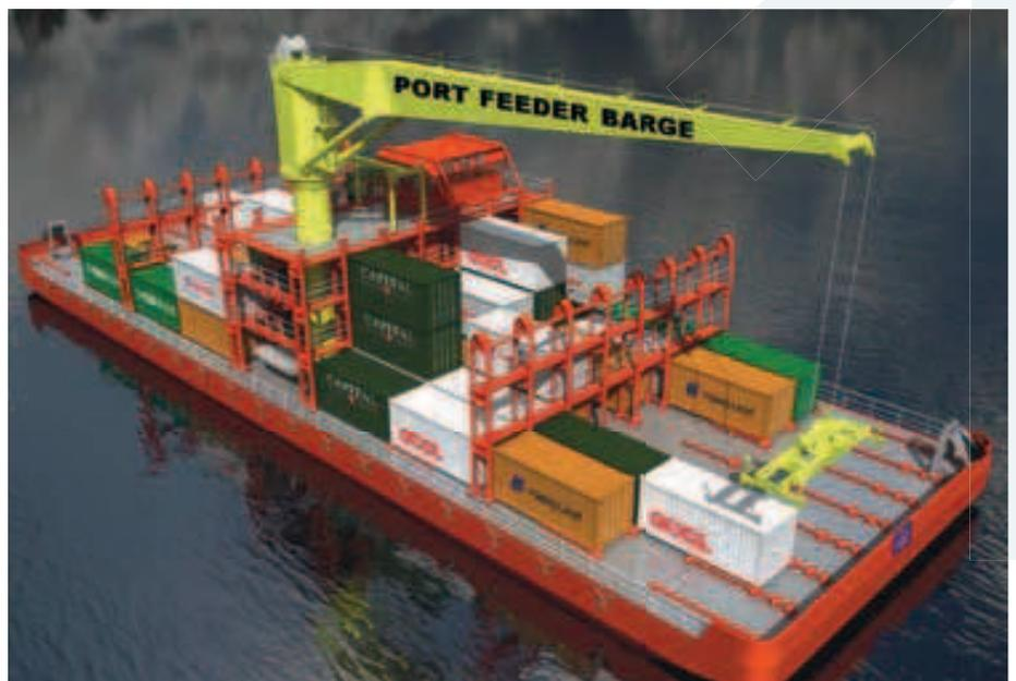
pick up the increasing number of container flats with out-of-gauge cargo. The crane has a capacity of 40 tonnes under the spreader at an outreach of 27 metres.
