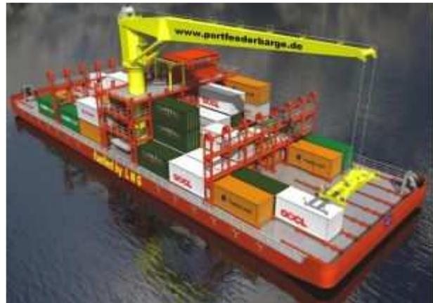
To make the barge self sufficient a Liebherr crane is installed on the opposite side of the superstructure to the control station
