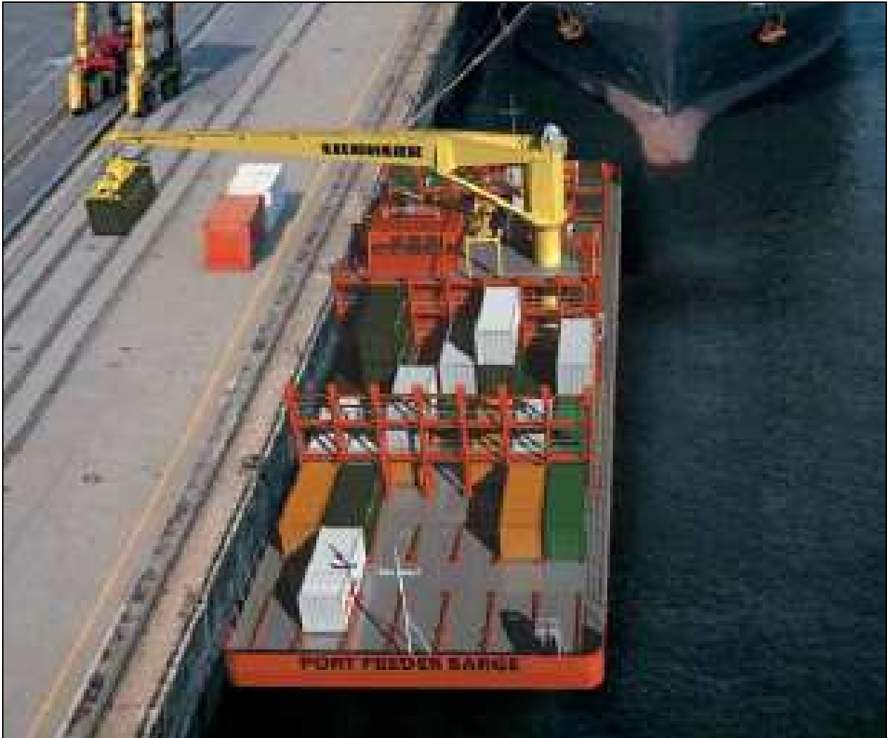
Fig. 4: Port Feeder Barge working independently from quayside equipment at a deep sea terminal requiring only a small gap between two deep sea vessels
